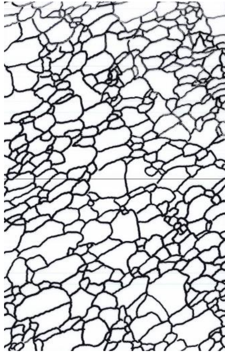
Figure A.4 Transparency used to calculate grain size of Haynes 230 at 800 °C
